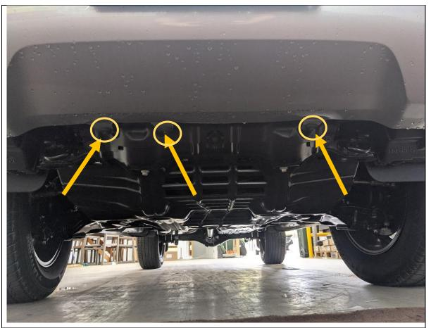
12. Remove the 3x 10mm head Screws securing bottom center section of bumper to inner wheel arch liner.
