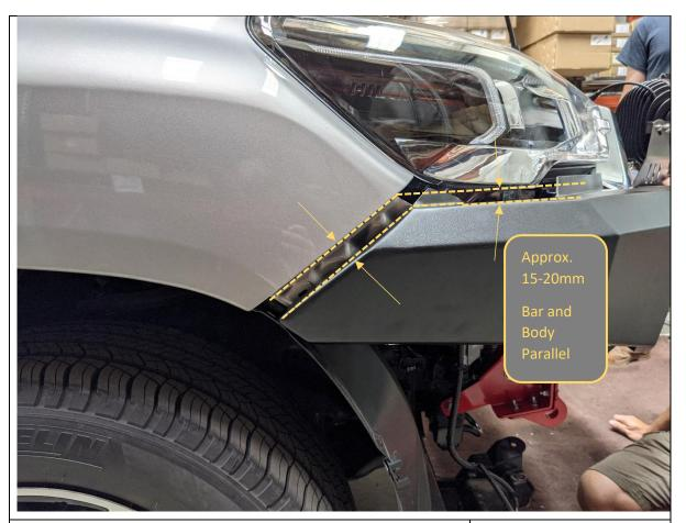
99. Align the bar with the body. Aim for 15-20mm clearance between the wing and body.
