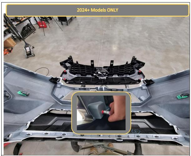
63. Separate grille from bumper by releasing the 4x Red clips. It can be helpful to push the clips from behind using a small socket to avoid marking the grille.
