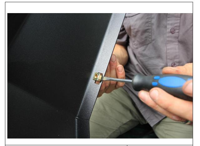
95. Insert cage nuts to square slots in bottom of wings.
