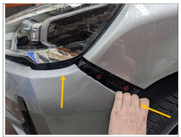
14. Remove the bumper. Start by pulling from the outside where the bumper meets the wheel arch and work towards the center from both sides.
