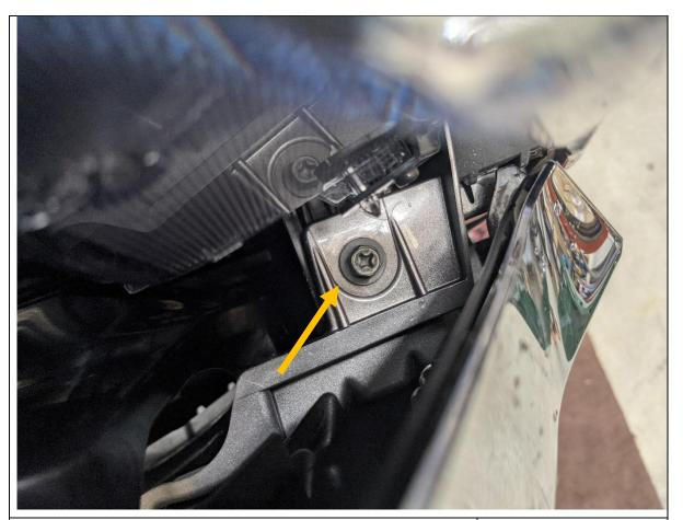
13. Remove the 2x 10mm Head/Phillips screws securing the bumper to crossmember.
