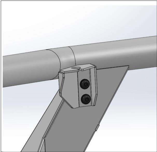
131. For Toro bars, if fitting antenna fit the antenna brackets to the captive nuts in the uprights using supplied M8x20 Button head bolts, and flat washers
