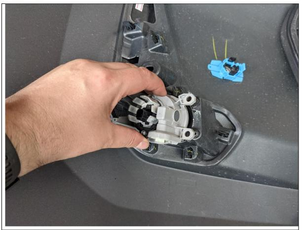
51. Remove the 3x Screws securing the fog lights to the bumper, then remove the fog light from the bumper
