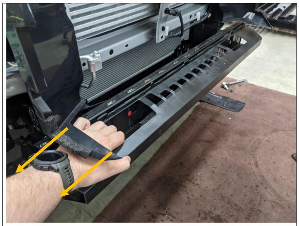
26. Remove the plastic cover from the impact beam by strongly pulling in the direction shown to release it from the clips
