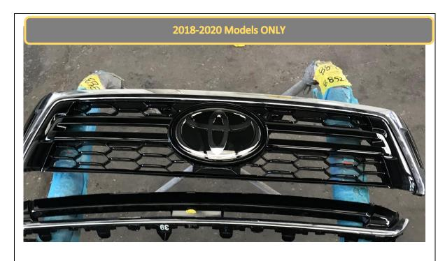
77. Using Similar technique as explained for 2021+ models cut the grille along the top edge of the horizontal bar below the badge, as shown in the above image.
