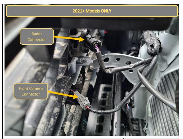
6. Unplug the radar sensor module wiring connector, located on the back of the Toyota Badge / sensor.
