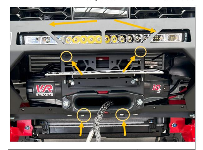
107. Fit Mesh panel to the bar. Ensure winch cable is fed through fairlead.
