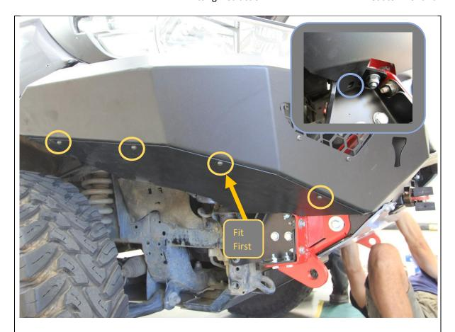
124. Fit side under panels to bar and secure with 4x M6x16 Button head bolts and M6 Flat washers, into M6 cage nuts fitted earlier.
